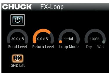
Let's rock the FX loop: With the "**FX Loop**" sub-page, you can control your parameters exactly as your sound requires. Here you even have the option of completely decoupling the **ground** of the FX loop - perfect if you have a second effect in the guitar signal that is also supplied by the **CHUCK**.
