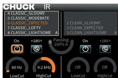
On this page you select your **speaker simulation**. You have an **A-** and a **B-side**, one of them must always be active. If you feel like it, you can activate both and mix the IRs with the **panning control**. With the  $-180^\circ$  switching surface, you can turn the phase on each side to suit your taste. There's also a **low and high cut** on each side to shape your sound perfectly.
